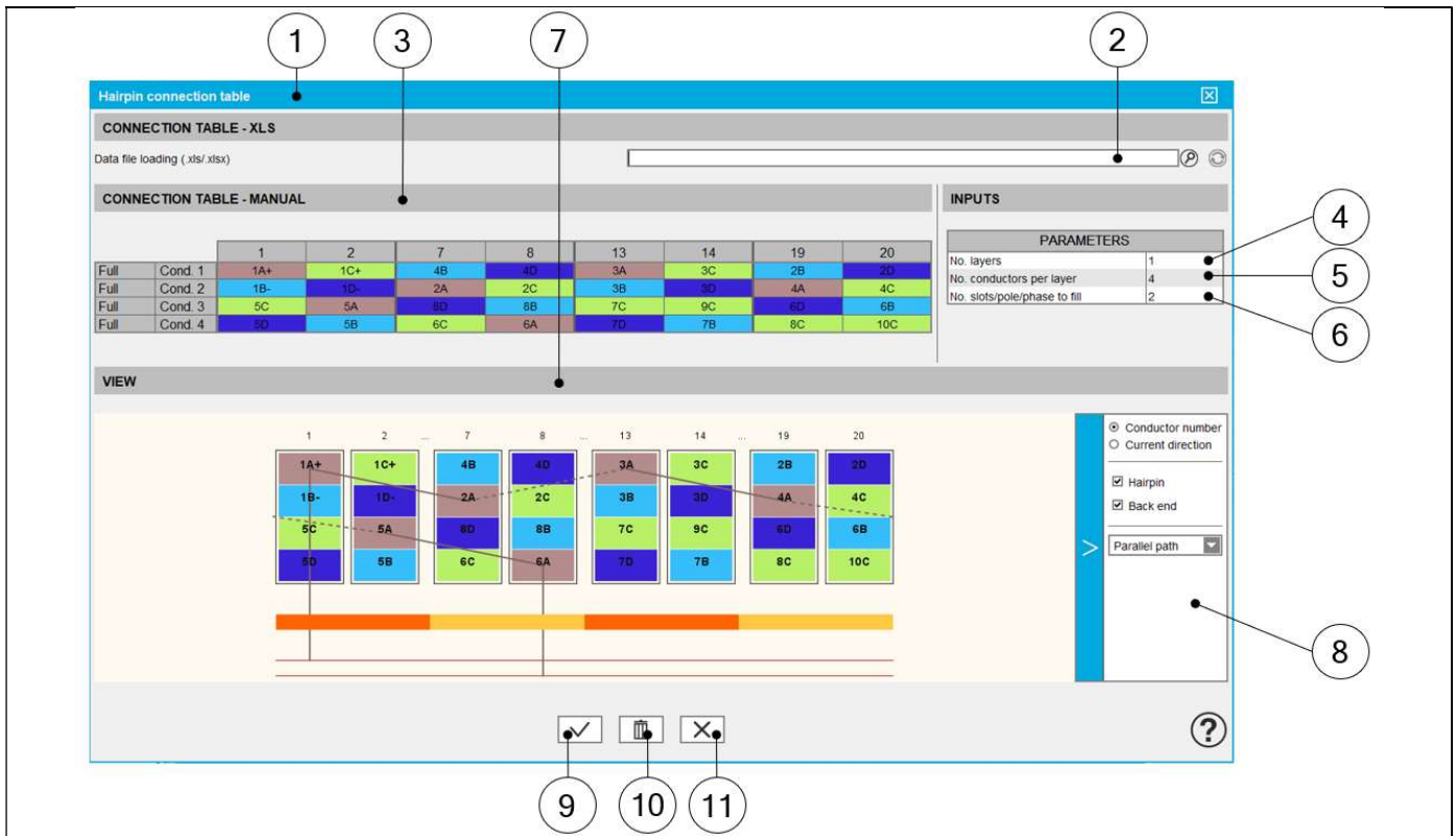
Building the winding architecture – Filling of the connection table
